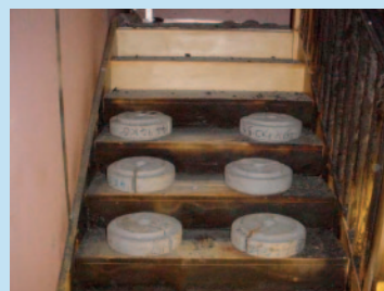
Protected stair after test
